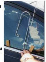
upper bend of the tool is inside the door, lower it until it is below the base of the window glass. As you work the tool up on the inside of the glass, watch the inside weatherstripping as you attempt to get the tool into position. As soon as you see the tool begin to bulge the weatherstripping upward, stop and remove the wedges.
