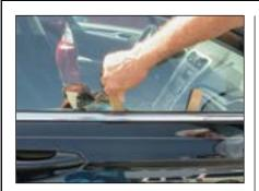
The first step is to wedge open a gap between the glass and the weatherstripping above the inside door handle. Here I'm using two wooden wedges inserted about eight inches apart, centered over the inside handle. Normally, I would use a shim, but on this occasion I didn't have one available so I carefully used the sharpest wooden wedges I had with me.
