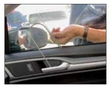
door with the inside handle; I'm trying to override the lock system. As soon as I feel the inside handle has been pulled out far enough, reach down with your other hand and pull the outside door handle. If you have the inside handle out far enough, this will open the door. Be prepared for the alarm to sound as soon as you open the door.
