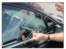
2 I'm using the Tech-Train 1015 tool, which is a pretty standard underthe-window tool. Almost any quality under window tool would work on the Fusion, but, as you will later see, you'll need a tool made from quality spring steel to get the leverage needed to unlock the door. Insert the tool between the wedges to attack the inside door handle.
